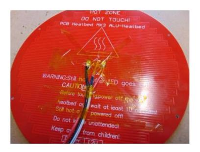
This completes the wiring for the heated bed
