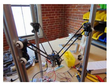
Slide the 'UPPER ASSEMBLY' on the top leaving about 20mm of the vertical 2020 beams sticking out.
