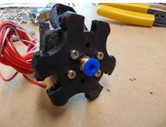
3. Once the hot end is attached we can now attach the inductive sensor. Make sure it fits before forcing it in, some sanding may be necessary.
