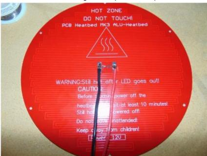
Once your solder joints are cooled off we are going to tape the end of the thermistor to the center of the printed side of the heat bed using Kapton Tape. The little glass ball is the temp sensor.
