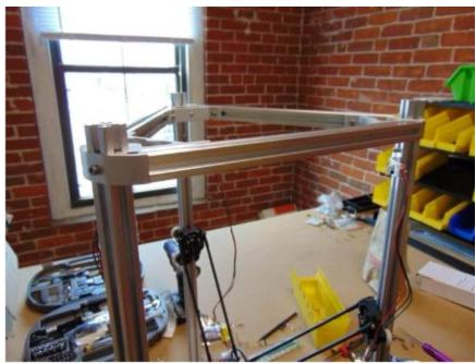
You can now install the endstops, making sure to place them an equal distance to the top of the beam. The distance you pick is not critical because this distance will be changed in the firmware during the configuration process.
