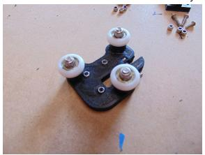
2. Insert 2 M3x20mm Bolts into the upper part of the carriage. Insert 1 M3x16mm Bolt into the lower part of the carriage
