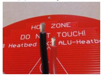
Solder one end of each wire to the two large solder pads on the printed side of the heat bed.
