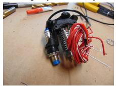
4. The probe should be mounted almost level with the print head using the 2 Jam Nuts supplied with the probe. Make sure the washers are sitting below the mount.
