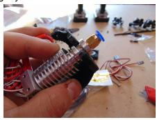
2. Once the hot end fits tightly into the mount we are going to attach the hot end to the End Effector using 4 M3x25mm bolts and 4 M3 Nylock Nuts.
