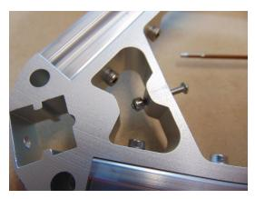
5. Using the two F623zz bearings face to face with the flanged side away from each other fit them onto the screw end allowing the screw to pass through them and continue into the other side of the corner as pictured.
