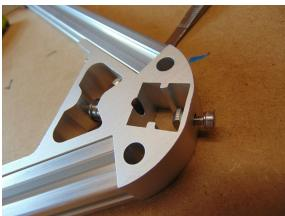
2. Once all the bolts are in place insert the 700mm 2020 Beams into the base assembly. Lock them in place securely using the bolt and T-Nut.
