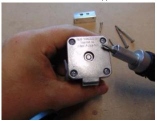
2. With the motor flat on the table and the connector facing you install the drive gear (with set screws sitting nearest the motor) and tighten the set screws on the drive gear to secure it to the motor shaft. Next install the Spring Loaded MK9, and Upper Aluminum Block in that order. Secure the Aluminum Block using 2 M3x20mm Bolts. Screw in the Push Fit as pictured below.
