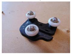
3. Insert the M3x20mm bolt through the side hole on the slider bracket and place the M3 Nut in the slotted opening in line with bolt and thread them together slightly. (This is the tensioner for the sliders that will be adjusted later.)
