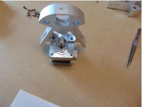
3. Using M4 T-Nuts and M4x10mm Bolts insert them through the side holes of you corner brackets as pictured. These will be used to secure the 2020 beam to the corners.
