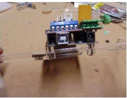
Once the ramps and mega are secure, prep the mount for installation into the frame by putting 4 M3x12mm Bolts into the corners of the mounting frame and securing them with M3 T-Nuts. Make sure your boards are facing downward.
