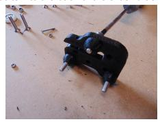
2. Once the bolts are in place, put the wheels on to the end of each M5 bolt, then secure in place using the the M5 Nylock Nut (It is a good idea to not tighten down on the nut too much as it may impede motion of the roller).
