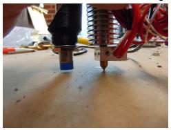
5. Using 2 M3x12 bolts, mount the Cooling Fan to the Hot End mount so the wires are at the top. The effector is complete, we now need to attach the diagonal rods.
