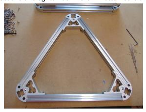
4. Next gather the 3 M3x25mm Bolts, 2 F623 Bearings, and 3 Nylock Nuts. Insert the bolt in the hole in the center point of the corners. Using a pair of plyers or a wrench thread the nylock nut partly onto the end of the M3 bolt that is coming through the back side of the corner so that you have a small amount of thread sticking out.
