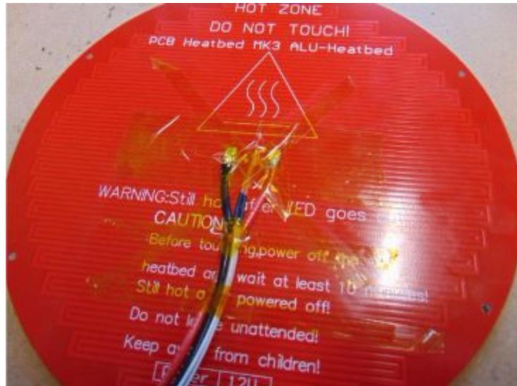
This completes the wiring for the heated bed
