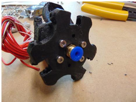
3. Once the hot end is attached we can now attach the inductive sensor. Make sure it fits before forcing it in, some sanding may be necessary.
