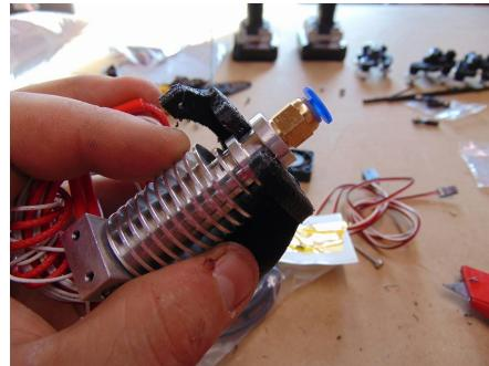
2. Once the hot end fits tightly into the mount we are going to attach the hot end to the End Effector using 4 M3x25mm bolts and 4 M3 Nylock Nuts.
