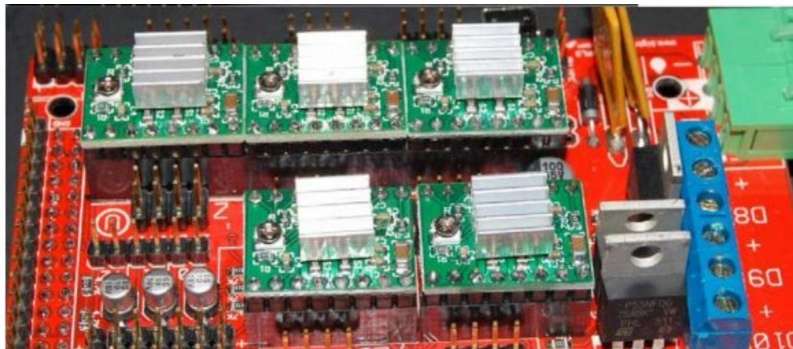
Align the pins and sandwich Ramps and Mega Boards, be sure they are tight and secure.
