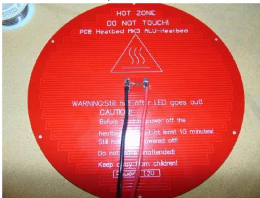
Once your solder joints are cooled off we are going to tape the end of the thermistor to the center of the printed side of the heat bed using Kapton Tape. The little glass ball is the temp sensor.
