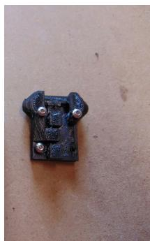
3. Line up the Belt Carriage with the Slider Assembly so the bolts line up with the bolt holes. You can now attach the carriage to the slider as pictured
