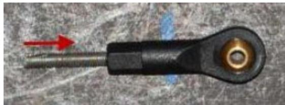
Measure the distance (in mm) from the end of the ball link to the center of the bolt hole and write it below.
